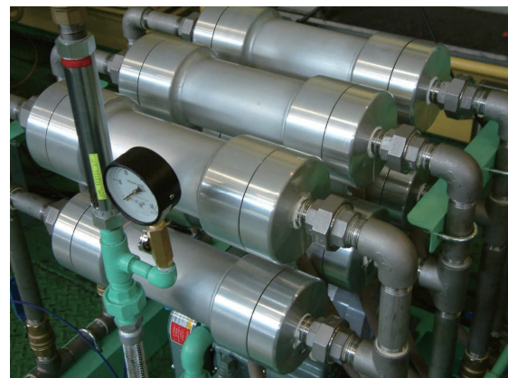
(a) Carburizing gas regenerator (b) Control panel Fig. 5 Appearance of “carburizing gas regenerator”.
