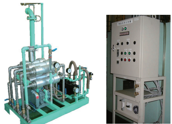
(a) Carburizing gas regenerator (b) Control panel Fig. 5 Appearance of “carburizing gas regenerator”.
