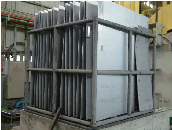
Fig. 7 Loading method of carburized quenching test.
