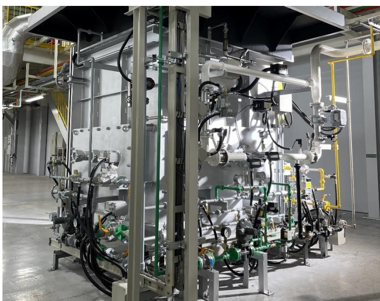
Entity Heating Demonstration Furnace that allows users to observe hydrogen combustion up close
