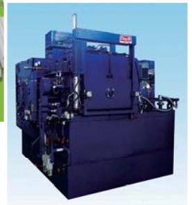
Furnace for validating small-lot vacuum carburizing
