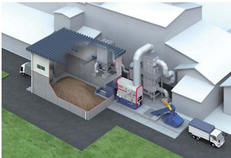
Image of wood biomass air-heating furnace in client's plant
