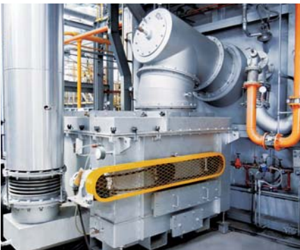
Aluminum melting furnace dedicated regenerative burner
