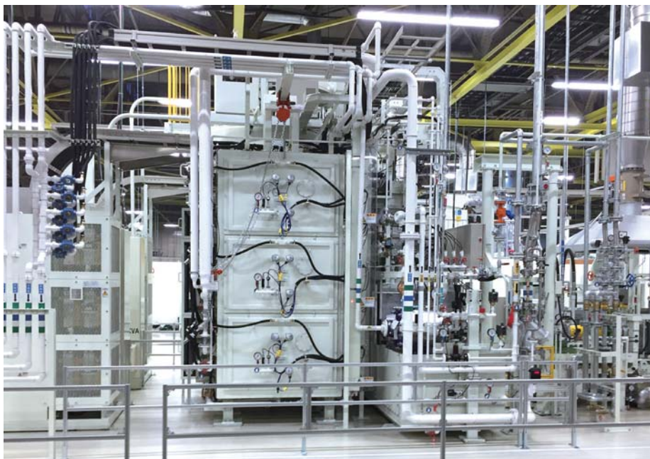
COMPACTFALCON™ small-lot type vacuum carburizing furnace
