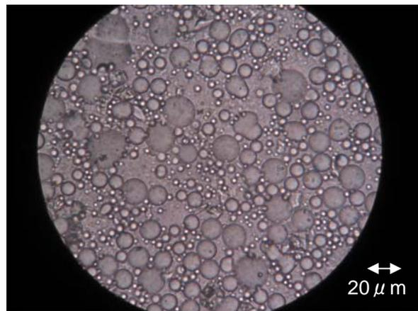
FIG. 10 Optical microscope photo of the powder material (Sample No. 2[Silica], magnification: 1000)
