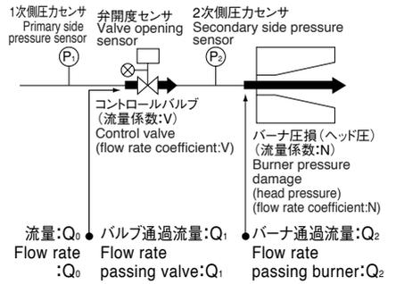
$$Q_1 = V \sqrt{P_1 - P_2} \dots\dots\dots ①$$
