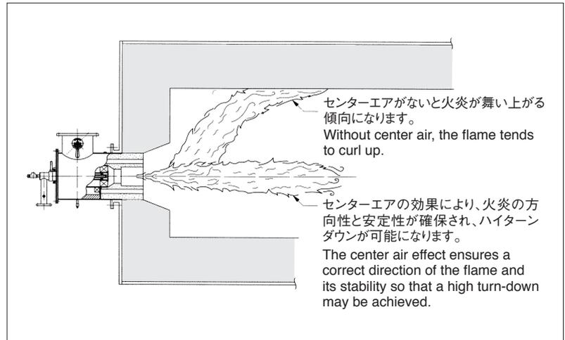
As the gas burner load is decreased, the flow rates of fuel gas and combustion air lower at the nozzle, causing insufficient mixing and thus resulting in poor combustion. To solve this problem, the "center air" system has been developed. This supplies a very small amount of air at a constant pressure.
