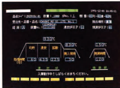
Incoming workpiece information If the name and quantity of workpieces are input when they are transferred into the warehouse, the transfer route, heating pattern, etc. are displayed.
