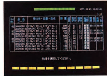
Detailed daily report Detailed production data of processed workpieces are displayed in order of treatment or for every furnace.
